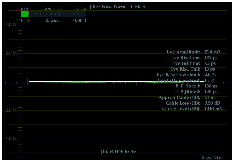
Figure 31: The Jitter display parameters as shown when the instrument is in single-tile mode
